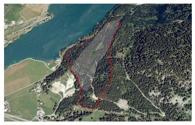
Figure 2: Aerial map of CH-Dav and proposed spatial features. The grey area represents the originally agreed TA (surface is 8.88 Ha, with a total excluded area is of 0.79 Ha. In a later stage, the TA was extended and agreed in order to better envelop the footprints in all the atmospheric conditions.
