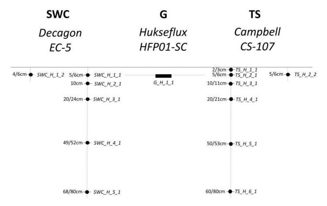
Figure 9: Set-up of the five soil plots (H = 1 to 5). SWC = volumetric soil water content, G = soil heat flux density, TS = soil temperature. X/Ycm indicates per sensor the variation in installation depth between the five plots.
